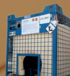
Large and bulky scraps such as stamping scraps can be transported in iron barred boxes (volume approx. 500 litres)
