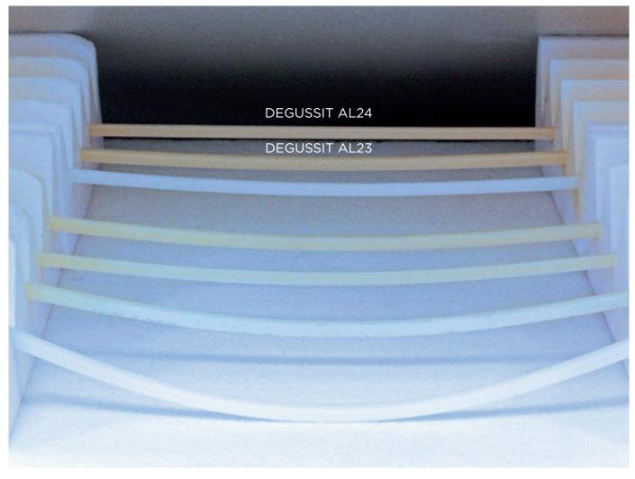
Comparative test used to determine  $\mathrm{Al_2O_3}$  high-temperature strength
